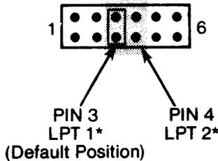
\*LPT 2 and LPT 3 respectively when the IBM Monochrome Display Card is installed
