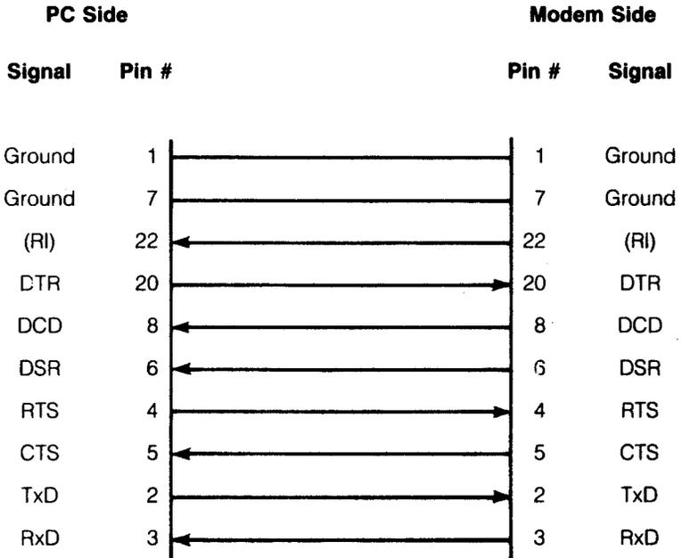
**Figure C-1. Ideal Case: DTE to DCE Interface**
