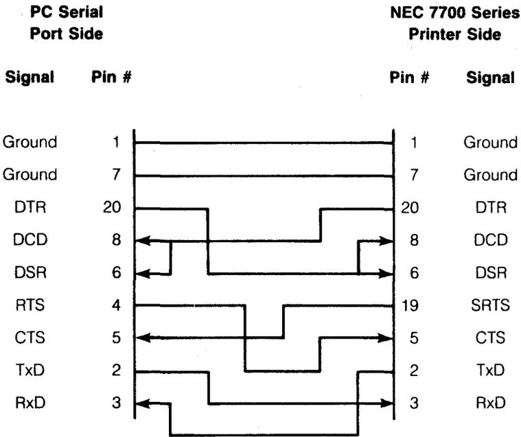
**Figure C-3. DTE to NEC 7700 Printer Interface**
