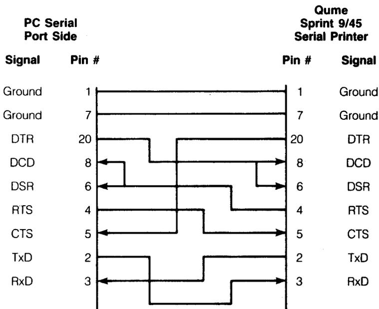
**Figure C-2. Typical (Non-Ideal) Case: DTE to DCE Interface**
